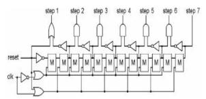
When we turn 'reset' on, it makes the input to the first 'M' bit a zero, and turns on all of the 'sets' at the same time so that the zero can travel down the line of 'M's very quickly. Reset is also ORed with step 1 so that step 1 turns on immediately. Now all of the bits are off, and we have started another sequence. Reset only needs to be turned on for a fraction of one clock cycle.
