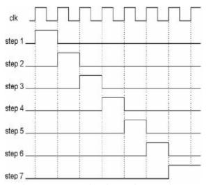
Here is how the stepper is built. It is done using some of the same memory bits that we used to make registers, but they are arranged very differently. We are not going to store anything in these bits, we are going to use them to create a series of steps.
