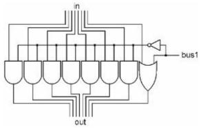
Now we can put this 'bus 1' and the ALU into the CPU. We will change where the wires go in and out of the ALU so it fits our diagram better. The bus inputs come in the top, the bus output comes out the bottom and all of the input and output bits are on the right.
