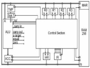
Below is the wiring within the Control Section that does the 'fetch' part of the instruction cycle. It uses the first three steps of the stepper and is the same for all types of instructions.
