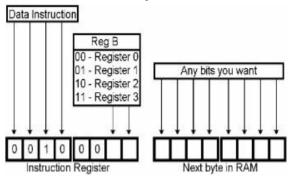
All this instruction needs to do is, in step 4, send IAR to MAR, and in step 5, send RAM to the desired CPU
