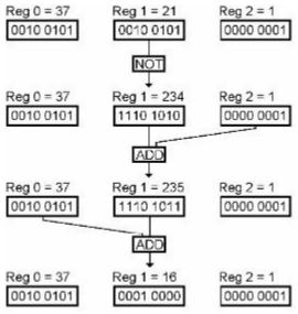
The last step is adding 37 + 235, the answer of which should be 272. But a single register cannot hold a number larger than 255. Therefore the adder turns on its Carry bit, and the eight bits remaining of the answer are 0001 0000, which is 16, the correct answer for 37 minus 21.
