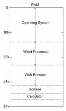
Within each program's RAM, there is all of the instruction code that makes the program work. Each program may be divided up into its own main loop, and many routines that are used for the various tasks that it needs to do. As mentioned, the OS also has routines that can be called by other programs.
