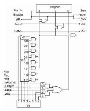
Step 4 moves IAR to MAR so we are prepared to get the 'Jump to Address' that we will use IF we jump. But because we might not jump, we also need to calculate the address of the next instruction in RAM. And so step 4 also turns on Bus 1 and sets the answer in ACC.
