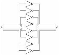
Since the input and the output are both eight wires, we'll simplify by using our bus type picture.
