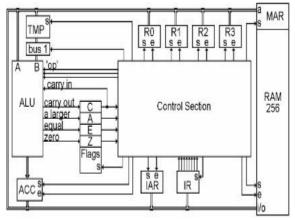
Here is the last register that we are going to add to the CPU. This will be called the FLAG register, and we are only going to use four bits of it, one for each of the flags.
