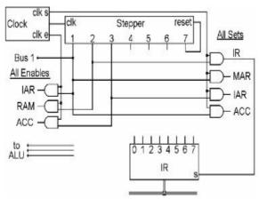
The stepper's first three steps are shown here, and result in 'fetching' the next 'instruction' from RAM. Then the rest of the steps 'execute' the 'instruction.' Exactly what will be done in steps 4, 5 and 6, is determined by the contents of the instruction that was fetched. Then the stepper starts over, fetches the next instruction, and executes it.
