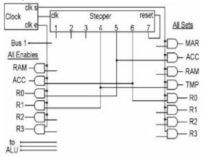
All we have to do to 'do something useful,' like adding Rl to RO, is to connect a few wires in the middle, as shown in this diagram with steps four, five and six. Each step causes something to happen to some of the parts that are shown in the CPU diagram. Each step is connected to one 'enable' on the left, and one 'set' on the right, and therefore causes one part to connect its output to the bus, and another part to save what now appears at its input. Step four is wired to Rl 'enable'
