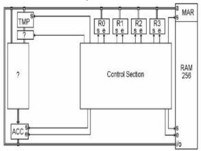
Here are the beginnings of the CPU. The RAM is shown on the right, and the bus makes a big loop between the two bus connections on the RAM. The CPU starts with six registers connected to the bus. These six registers are all of the places that the CPU will use to "process" bytes. That's not so complicated, is it?
