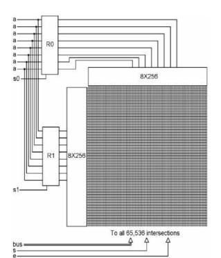
A bus carries one byte at a time, so selecting one of the 65,536 memory locations of this RAM would be a two-step process. First, one byte would have to be placed on the 'a' bus and set into RO, then the second byte would have to be placed onto the 'a' bus and set into R1. Now you could access the desired memory location with the bus and the 's' and 'e' bits at the bottom of the drawing.
