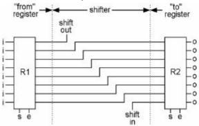
Once again, we have bus versions of these drawings. They each have an 'i' and 'o' bus, and also one input and output bit, like this:
