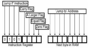
Here is the wiring in the Control Section that makes the Jump If instruction work.
