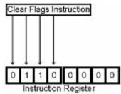
The wiring for this is very simple and a bit tricky. We will not enable anything onto the bus, thus it and the '^A' ALU input will be all zeros. We will turn on 'Bus 1'.
