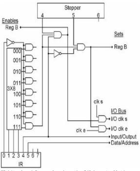
IR bits 4 and 5 are placed on the I/O bus at all times.
