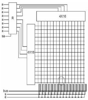
At the bottom of this diagram is one bus and an 's' and 'e' bit, just the same as the connections that go to a register. As you can see, they go upwards and into the grid. The diagram doesn't show it, but they go up under
