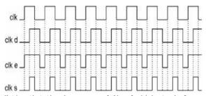
Notice that they have names, 'clk e,' which stands for clock enable, and 'clk s,' which stands for clock set. And what do you know, these two bits have the perfect timing to move a byte of data from one register, across the bus, and into another register. Just connect 'clk e' to the enable bit of the 'from' register, and connect 'clk s' to the set bit of the 'to' register.
