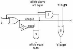
If the output of gate 1 is on, that means that 'a' and 'b' are different, or unequal. We add gate 2, which will turn on when 'a' and 'b' are equal.
