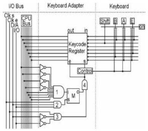
After pressing a key, there will be an ASCII code waiting in the Keycode Register. Here's how the CPU gets that code into one of its registers.
