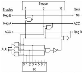
IR bit 0 continues up the diagram, turns right and is connected to one side of three more AND gates. The other sides of these gates are connected to Steps 4, 5 and 6.
