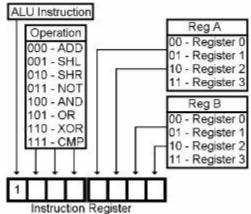
Therefore, the ALU Instruction (1), to add (000) Register 2 (10) and Register 3 (11), and place the answer in Register 3, would be: 1000 1011. If you placed this code (1000 1011) in RAM at address 10, and set the IAR to 10, and statted the computer, it would fetch the 1000 1011 from address 10, place it in IR, and then the wiring in the control section would do the addition of R2 and R3.
