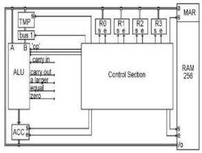
The output of the ALU is connected to ACC. ACC receives, and temporarily stores, the result of the most recent ALU operation. The output of ACC is then connected to the bus, so its contents can be sent somewhere else as needed.
