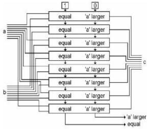
Simplifying again, we will go back to the bus-type XOR diagram, and just add the two new output bits of the comparator.
