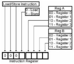
The Instruction Code for the Load instruction is 0000, and for the Store instruction is 0001. The remaining four bits in both cases specify two registers, just like the ALU instruction did, but in this case, one register will be used to select one of the locations in RAM, and the other register will either be loaded from, or stored to, that RAM location.
